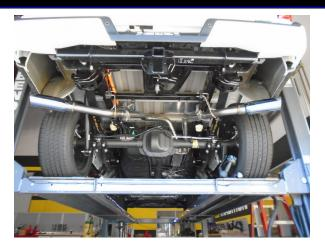
**Step 6.** Once a final position has been chosen for the new exhaust system, evenly tighten all clamps from front to rear using the torque specifications on page one of the instructions. Inspect all fasteners after 25-50 miles of operation and re-tighten if necessary.
