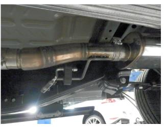
**Step 2.** Begin installing the new system by first using *Table 1*. to determine which Inlet Pipe Assembly to use for your vehicle. Once determined attach the Inlet Pipe Assembly to the OEM catalytic converter outlet pipes using the existing clamp and hardware. Locate the welded hanger to the rubber insulator. Leave all clamps and fasteners loose for final adjustment of the complete system once installed.
